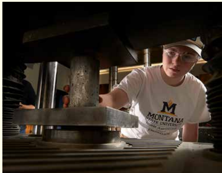
Students in the structures laboratory perform concrete strength testing.
