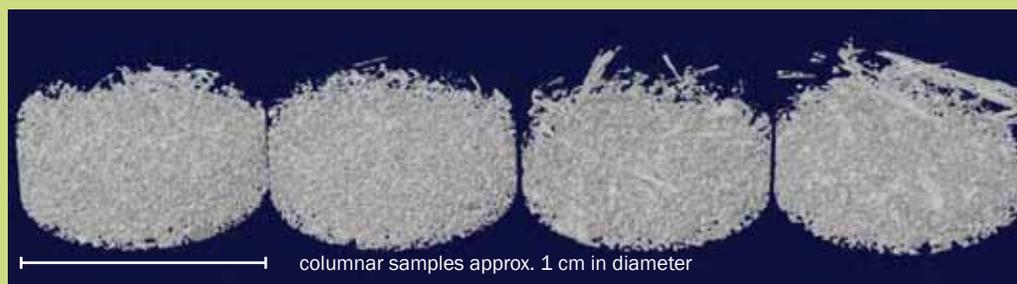
This series of micro-CT scanner images of a snow sample shows the progression of radiation recrystallization from left (none) to right (fully developed).
